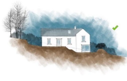
Fig. 13.9 Reduce cutting and filling in sloping sites by making floor levels work with existing topography and contours.
