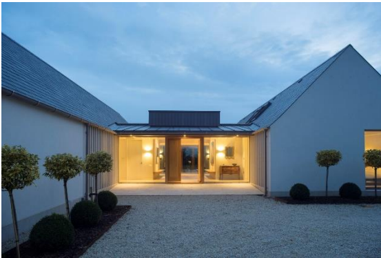
Fig. 13.21 – The transparency of some forms helps in the definition of the massing of each block. It also helps to establish a relationship with the landscape (Tierney Haines Architects)
