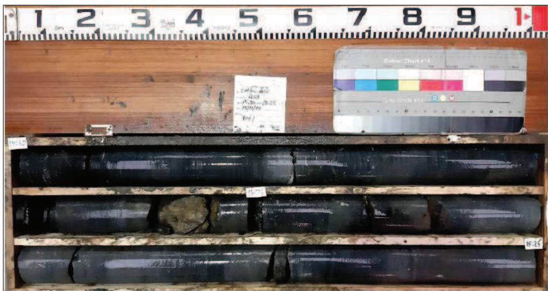
Photo 1 – Core recovery at RC03 (15.3 to 18.25 m)
