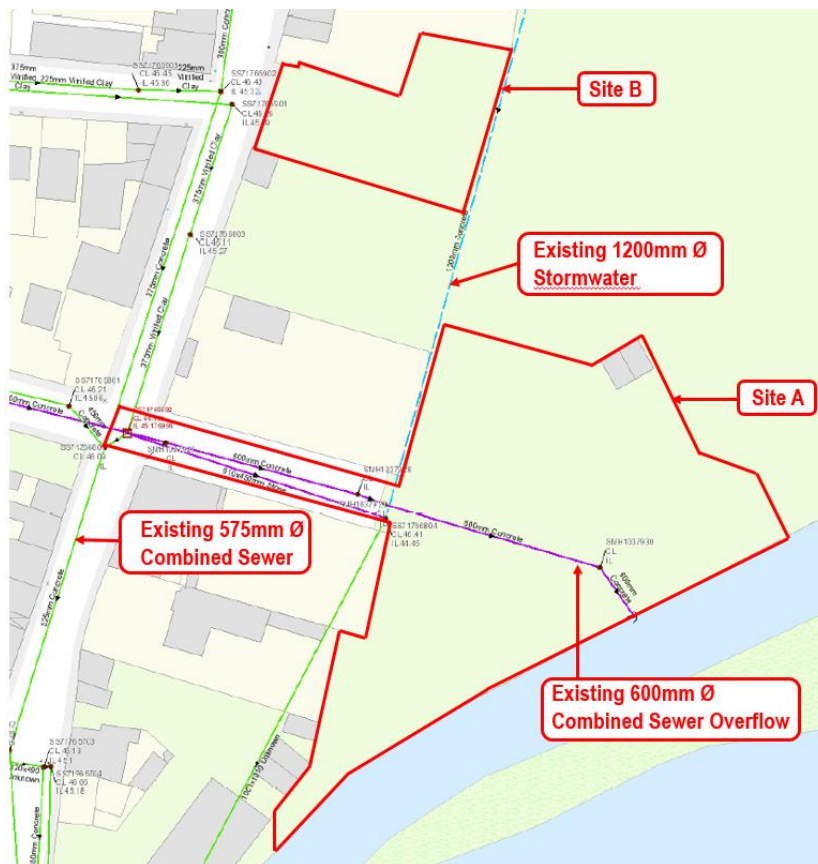
Figure 4 – Extract from Irish Water Wastewater Services Map
