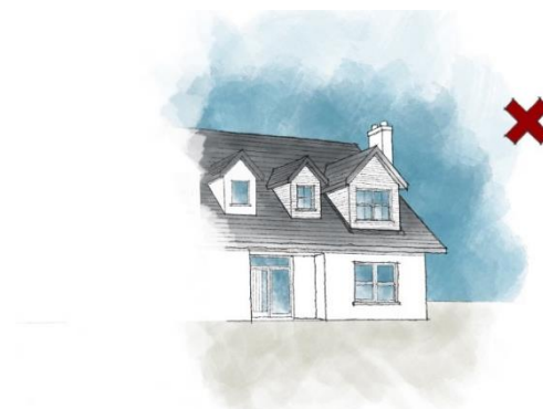
Fig. 13.24 Avoid box verges and eaves and the use of cladding. Ideally dormer windows should be connected to the façade as in Figure 13.22 and not be protruding separately from the roof.
