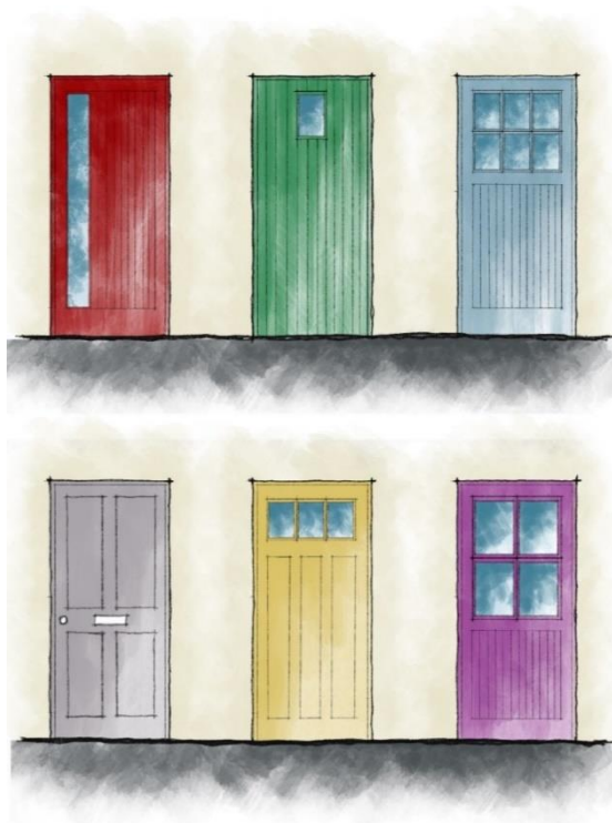
Fig. 13.34 Appropriate simple design panelled and sheeted doors.
