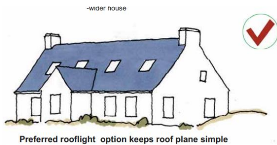
Fig. 13.26 Use of Alternative approach to mid-roof dormers can be symmetrical rooflights to simply roof profile and reduce building scale.
