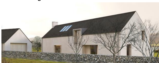
Fig. 13.27 This 1 ½ storey height helps reduce the mass of the building and potential proportion of the roof relative to wall area. There is also an example of a modern interpretation of the dormer window which is a much nicer detail than a typical mid-roof dormer. (Tierney Haines Architects)
