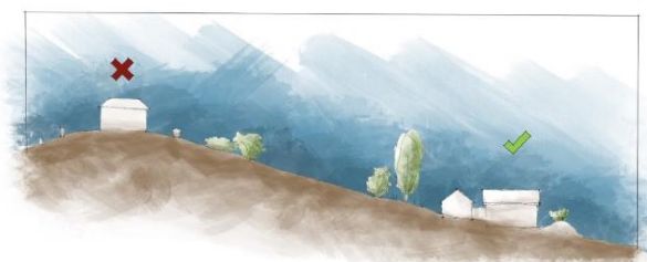
Fig. 13.7 A more appropriate approach is to site house on lower, more sheltered and less visually exposed ground.
