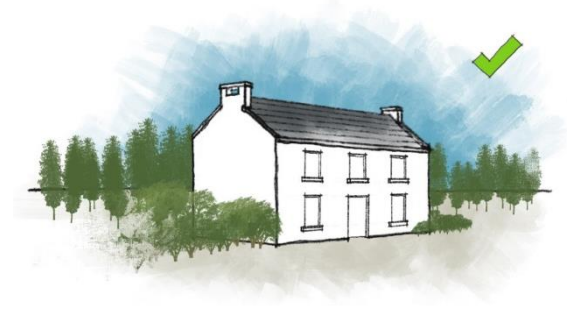
Fig. 13.31 Vertical emphasis windows and symmetrical arrangement.
