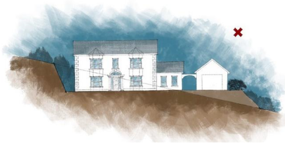
Fig. 13.8 Avoid excessive cutting and filling on sloping sites. This can leave landscape scarred and give impression house has been “dropped into” an area.
