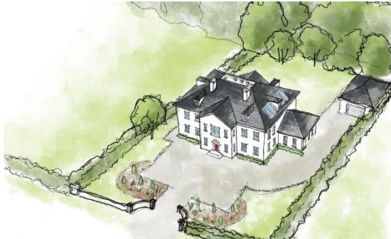
Fig. 13.10 Large house out of scale on a small site
