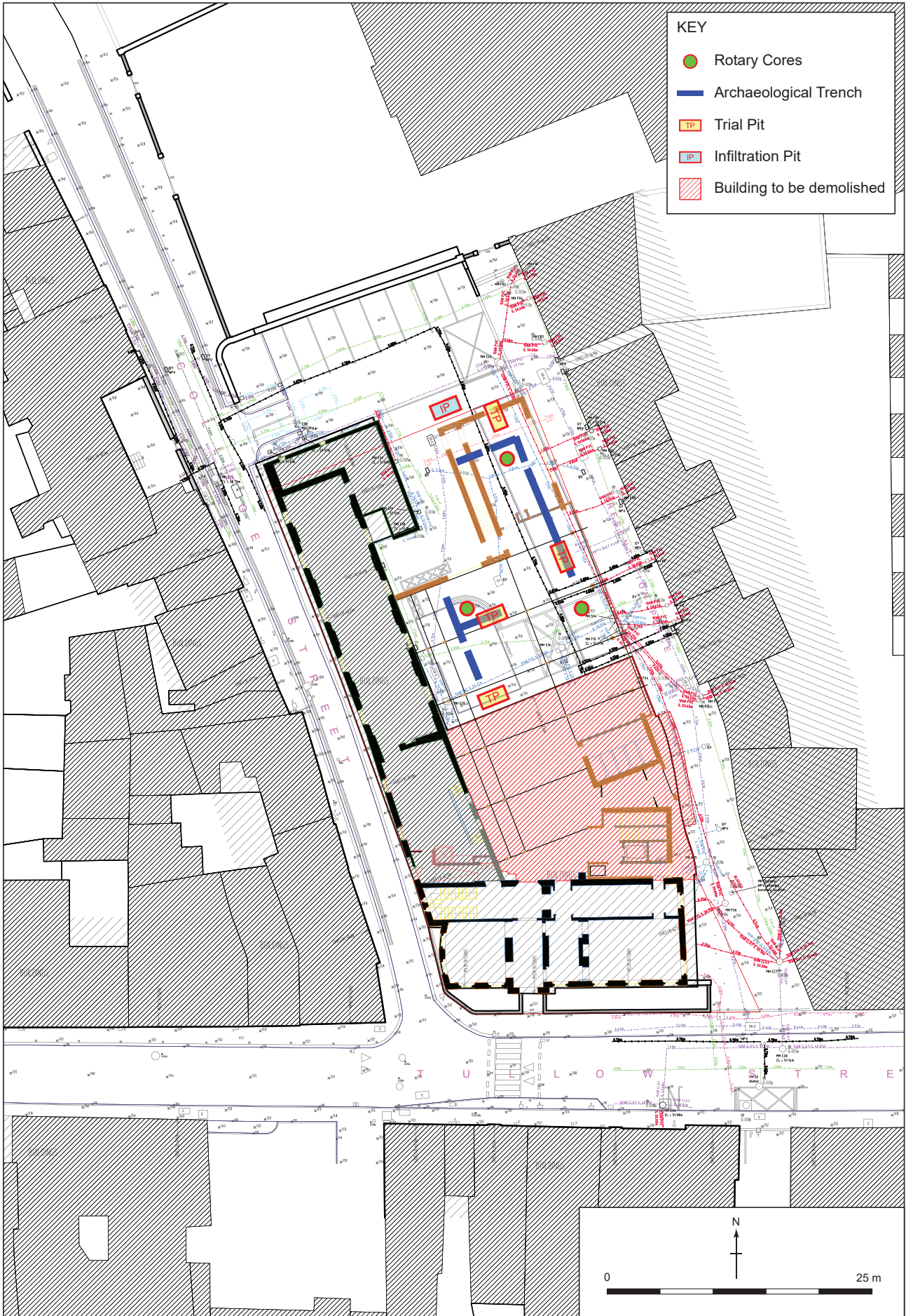
Figure 2 - Excavated test trench layout.
