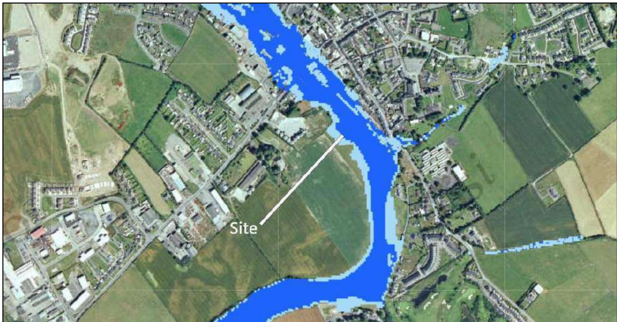
Figure 15 CFRAM flood extent (mid-range future)
