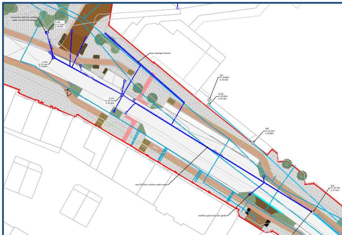
Fig. 4-1 New section of surface water sewer on Kennedy Avenue
